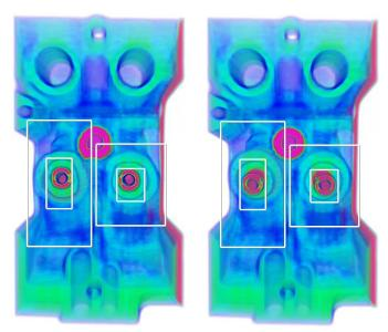
Fig. 5. Multiperspective volume rendering of a density engine block dataset (left) and conventional visualization (right), for comparison. In the multiperspective visualization the viewpoints of the two focus regions are adjusted to provide a visualization along the piston axes
