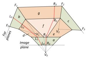
Fig. 7. Camera model that integrates two conventional images with viewpoints  $V_1$  and  $V_2$  into a multiperspective image. The green camera segments are implemented with conventional planar pinhole cameras. The orange camera segments are implemented with continuous general linear cameras. The rays are piecewise linear, e.g.  $L_0L_1L_2L_3$  and  $R_0R_1R_2R_3$ .
