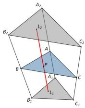
Fig. 8. Continuous general linear camera frustum. The endpoints  $L_1$  and  $L_2$  of ray  $L_1L_2$  have the same barycentric coordinates in triangles  $A_1B_1C_1$  and  $A_2B_2C_2$ . 3D point P projects at  $L_1$ .
