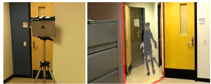
Fig. 3: Left: the RGB camera with depth sensor accessory captures a RGBD video stream that is converted to a 3D point cloud. Right: the point cloud, as seen from the secondary perspective, is integrated into the primary perspective in the multiperspersive visualization.
