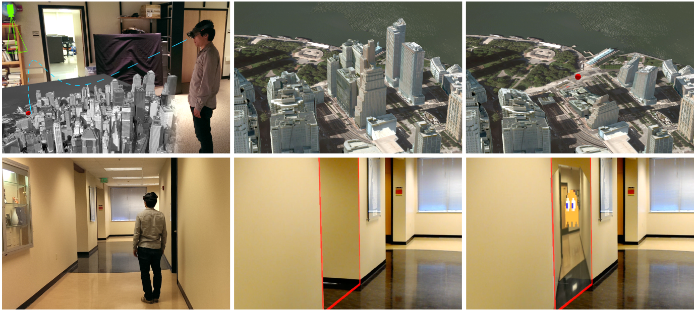
Fig. 1: (Top) Multiperspersive disocclusion in a VR exploration of an urban scene: artist rendition of a second-person view (left), conventional VR visualization (middle), and our multiperspersive VR visualization (right). The user does not have a direct line of sight to the red sphere, which is occluded in the a conventional image; an additional perspective (green frustum) is used to route rays over the occluding buildings (dashed blue line), which disoccludes the red sphere in the resulting multiperspersive image. (Bottom) Multiperspersive disocclusion in an AR exploration of a real world indoor scene: second-person image (left), conventional image from user viewpoint (middle), and our AR multiperspersive visualization (right). The left side corridor is disoccluded by inserting an additional perspective at the portal (red rectangle), which reveals the target (orange ghost).
