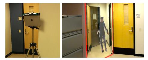
Fig. 3.3.: Left: the RGB camera with depth sensor accessory captures a RGBD video stream that is converted to a 3D point cloud. Right: the point cloud, as seen from the secondary perspective, is integrated into the primary perspective in the multiperspective visualization.
